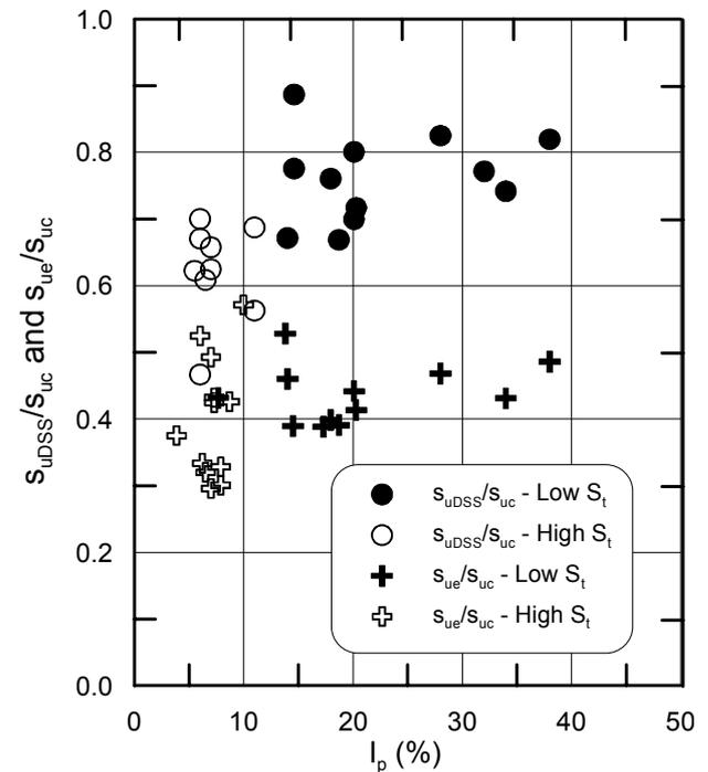
Figure 4. Measured anisotropic strength ratios  $s_{ue}/s_{uc}$  and  $s_{uDSS}/s_{uc}$  for the block samples
