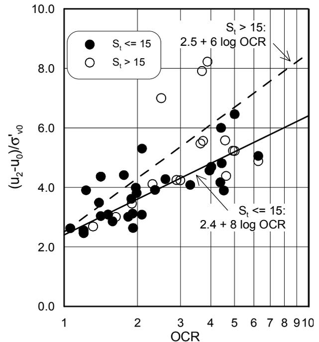
Figure 16. Relationship normalised excess pore pressure  $(u_2-u_0)/\sigma'_{v0}$  and OCR
