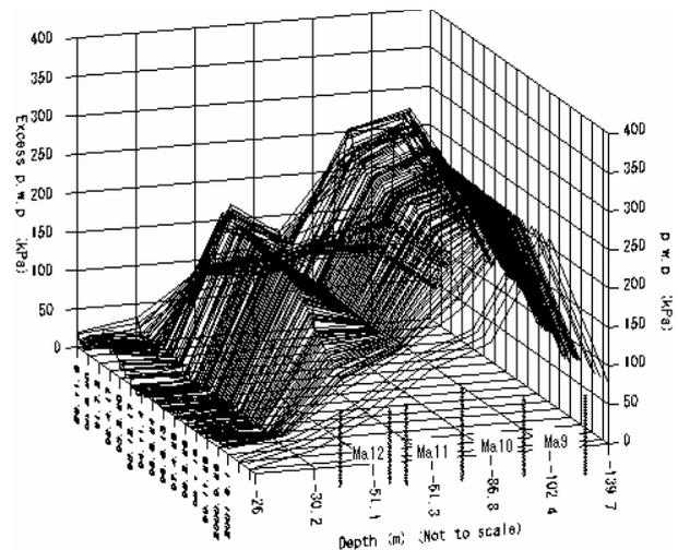
Figure 3. Excess pore water pressure distribution beneath the airport
