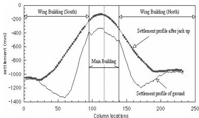
Figure 5. Settlement profiles of the Passenger Terminal Building along the longitudinal direction.
