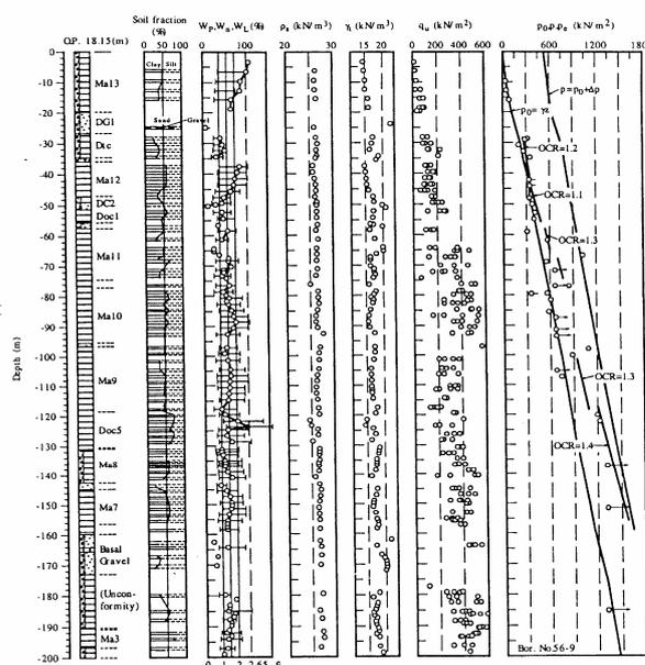
Figure 1. Typical geotechnical profile of seabed beneath the airport
