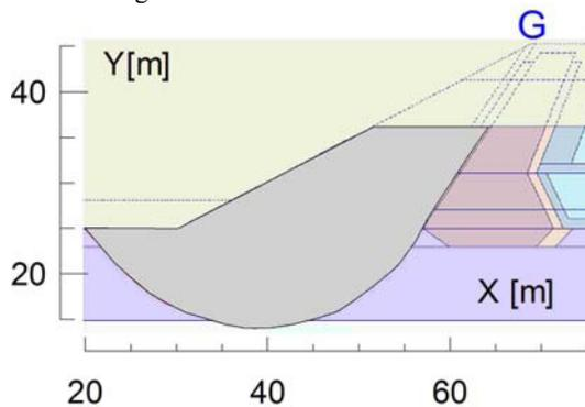
Figure 5. Results of the back-analysis of soil failure
