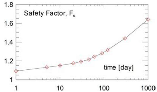
Figure 6. An increase in factor of safety depending on time of placement of the third fill layer.
