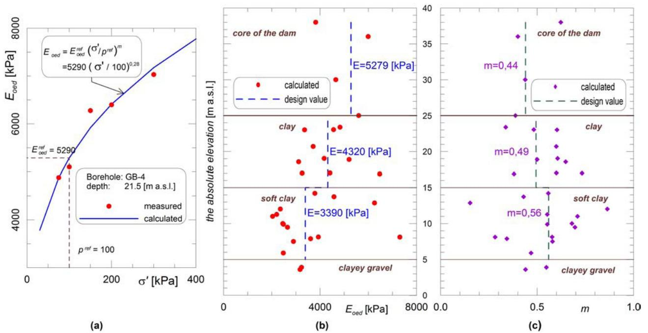
Figure 2. Deriving  $E_{oeod}^{ref}$  and  $m$  from an oedometer test (calculated values) (a); Calculated and design (average) values for  $E_{oeod}^{ref}$  (b), and  $m$  (c) through the dam core and the foundation soil profile.
