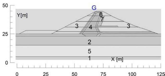
Figure 1. The characteristic cross-section of the Botonega dam used in numerical model (description of soil indicated by numbers are given in Tab. 1 and 2).
