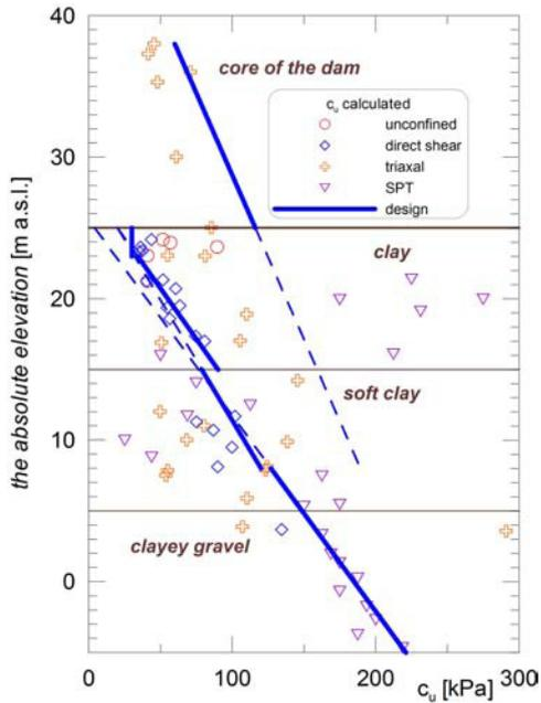
Figure 4. Comparative diagrams of in situ and laboratory tests for determination of undrained strength.
