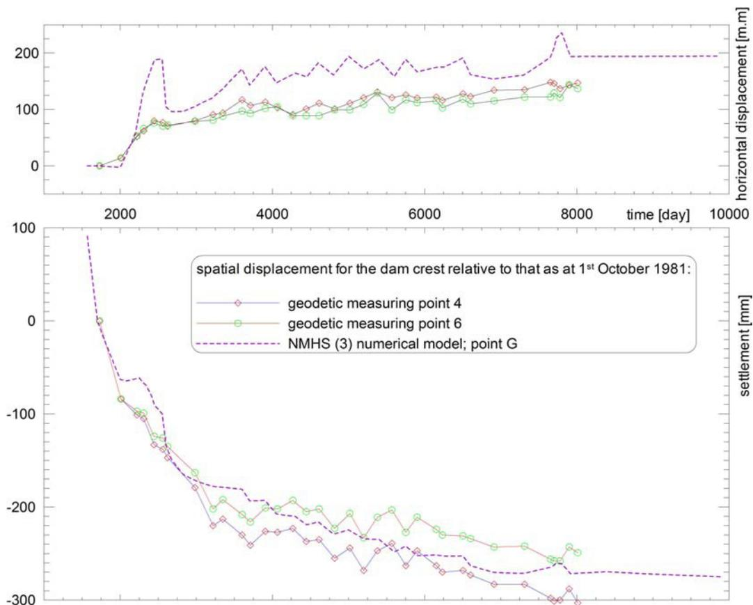
Figure 3 Comparative diagrams of horizontal displacements in transversal direction and settlements of the point G and of those at geodetic measuring points 4 and 6 at the crest
