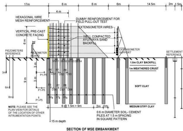
Figure 2b. Centerline elevation of Test Embankment.
