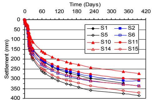
Figure 3. Surface settlement "on clay" and "on pile" (solid symbols=on piles; hollow symbols=on clay).
