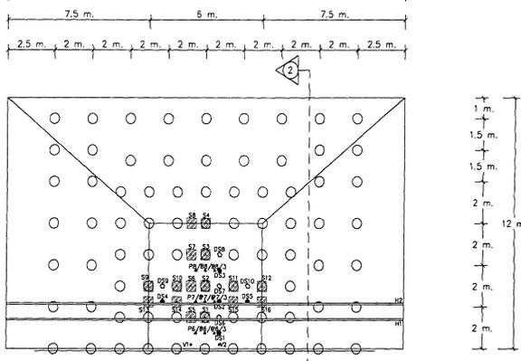
Figure 2a. Plan view of Test Embankment.
