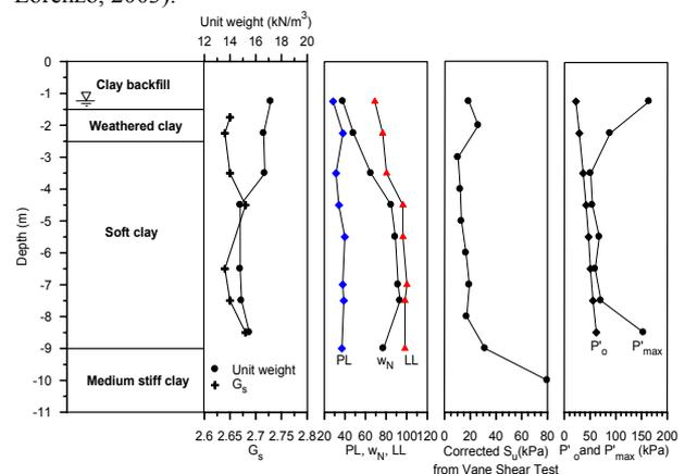
Figure 1. Soil profiles under the Test Embankment.
