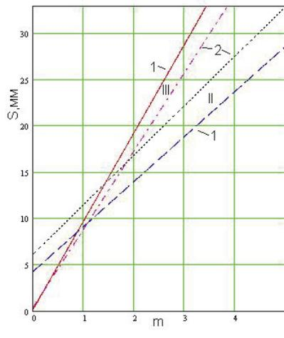
Figure 2. Comparison of buildings settlements  $S$  dependence on  $m$  for retaining structures fastening with buntions made of metal pipes for buildings of II and III structure category (1 – experimental dependences, 2 – calculated (PLAXIS, Brinkgreve and Vermeer, 1998) dependences).
