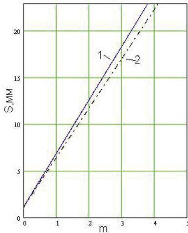
Figure 1. Comparison of experimental buildings settlements  $S$  dependence on  $m$  for retaining structures fastening with buntions made of metal pipes: 1 – for sheet piling made of metal pipes with wooden fencing, 2 – for “slurry walls” of different types.
