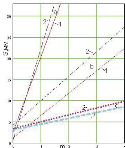
Figure 4. Buildings settlement  $S$  dependence on  $m$  (1 - experimental, 2 - calculated (with the help of PLAXIS [2] program)) for various types of foundation trench retaining structure fastening: a – with anchors, b – with buntions made of metal pipes, c – with reinforced-concrete floor structures (“top-down” method).
