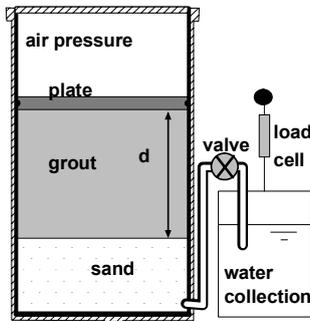
Figure 9. Grout consolidation, measurement principle.
