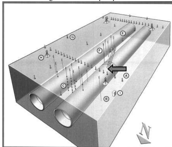
Figure 1. Artist impression measurement field 2<sup>nd</sup> Heinenoord Tunnel. The arrow indicates the pore pressure gauges in front of the TBM. Results of the gauge in the middle are used this paper. Drilling was from North to South (Bakker et al. 2003).
