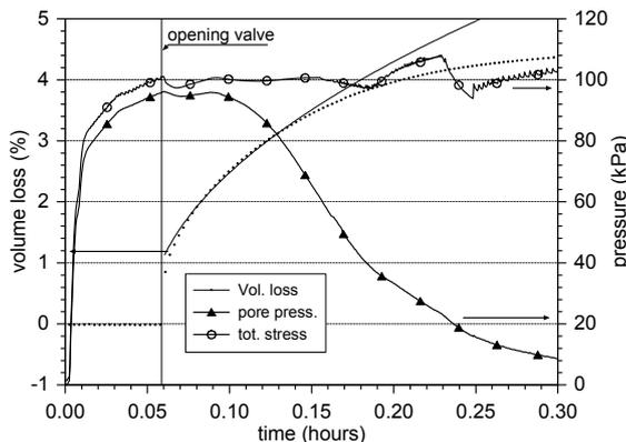
Figure 11. Result of consolidation test. Pore pressure and total pressure are measured on the impermeable plate.
