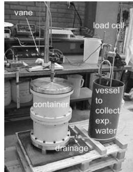
Figure 10. Grout consolidation, experimental setup.
