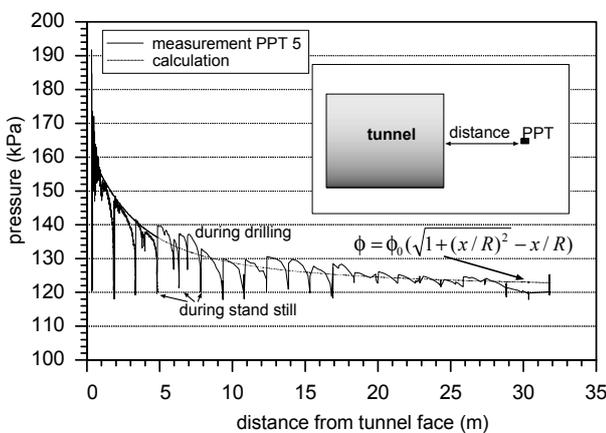
Figure 2. Measured excess pore pressure in front of a slurry shield and approximation.
