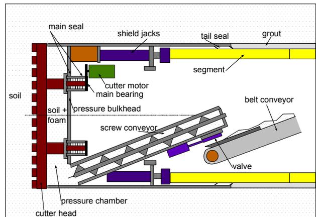
Figure 3. Principle of EPB TBM.
