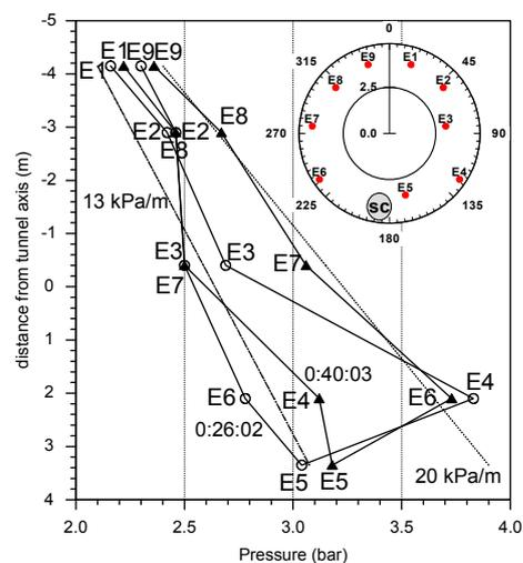
Figure 4. Example of non-hydrostatic pressure distribution measured at the Botlek rail tunnel. The rotation direction of the cutter head was reversed between the 2 measurements shown. The inset shows the position of the instruments and the position of the screw conveyor (SC) in the pressure bulkhead of the TBM.
