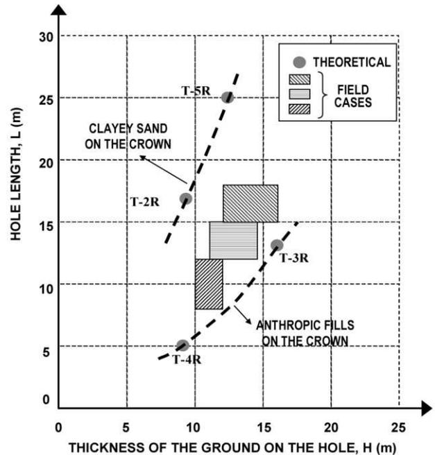
Figure 8. Comparison between PLAXIS-3D results and field situations.
