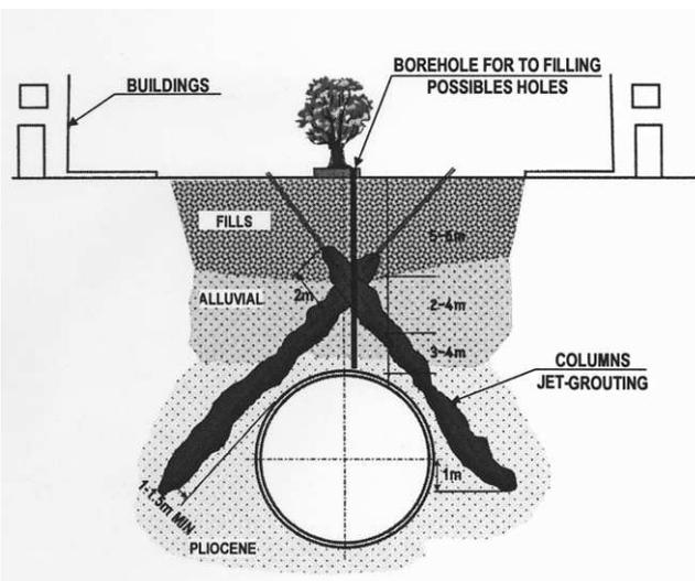
Figure 10. "Canadian tent" solution for frontal and dorsal tunnel instability (Oteo, 2003).
