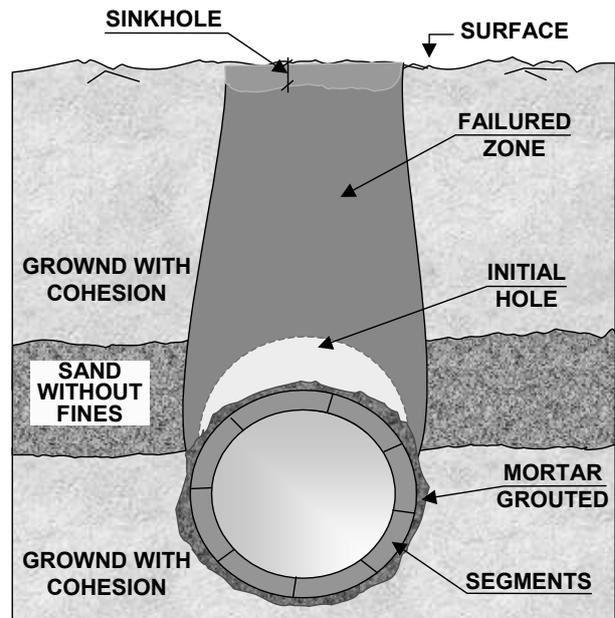
Figure 3. final dorsal instability (cross section).
