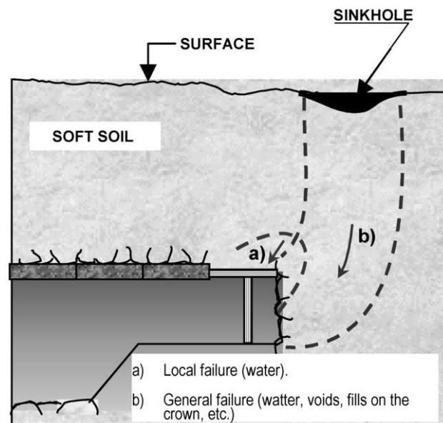
Figure 1. Lay-out of frontal tunnel instability.
