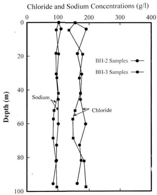
Figure 3. Chloride and Sodium concentrations in pore-water versus bore-hole depth, in BH-2 and BH-3 soil samples
