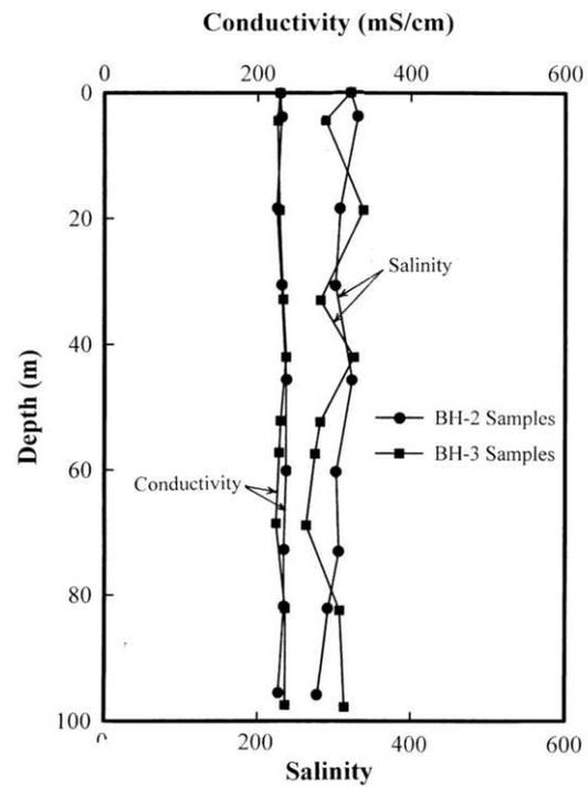
Figure 6. Salinity and conductivity values in pore-water versus bore-hole depth, in BH-2 and BH-3 soil samples
