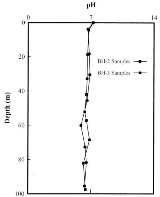
Figure 5. pH values in pore-water versus bore-hole depth, in BH-2 and BH-3 soil samples
