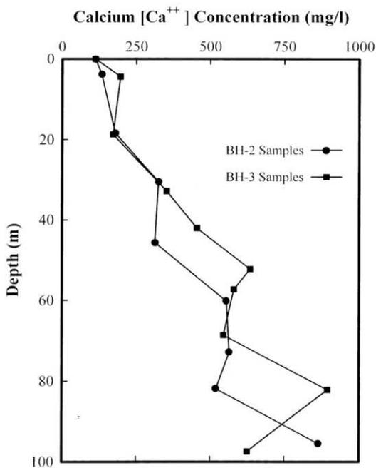
Figure 4. Calcium concentrations in pore-water versus bore-hole depth, in BH-2 and BH-3 soil samples
