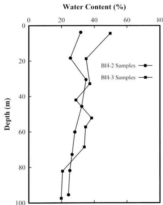
Figure 2. Water contents versus depth, in BH-2 and BH-3 soil samples
