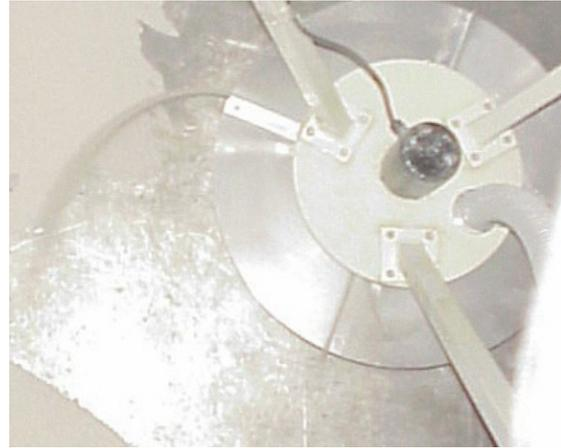
Figure 3. Spinning disk spreading sand in the ETHZ drum centrifuge (Laue et al., 2001).
