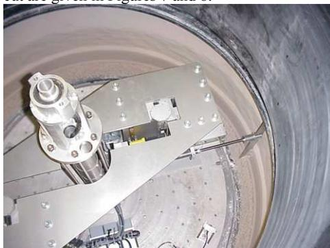
Figure 6: Scraping the model surface, view from the top of the centrifuge into the machine. The soil model is drum channel while the scraping tool is mounted into an actuator placed on the rotating toolplate.
