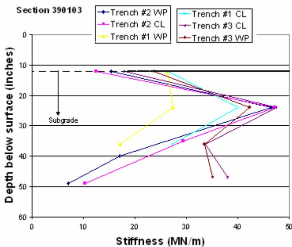
Figure 5. Humboldt subgrade stiffness of Section 390103
