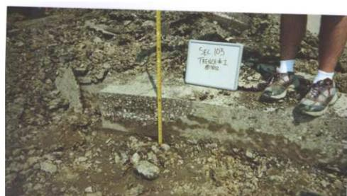
Figure 4. Measurement of lift layers at a trench
