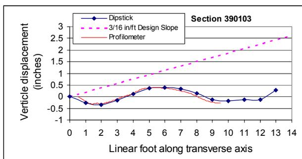
Figure 3. Transverse profile of Section 390103
