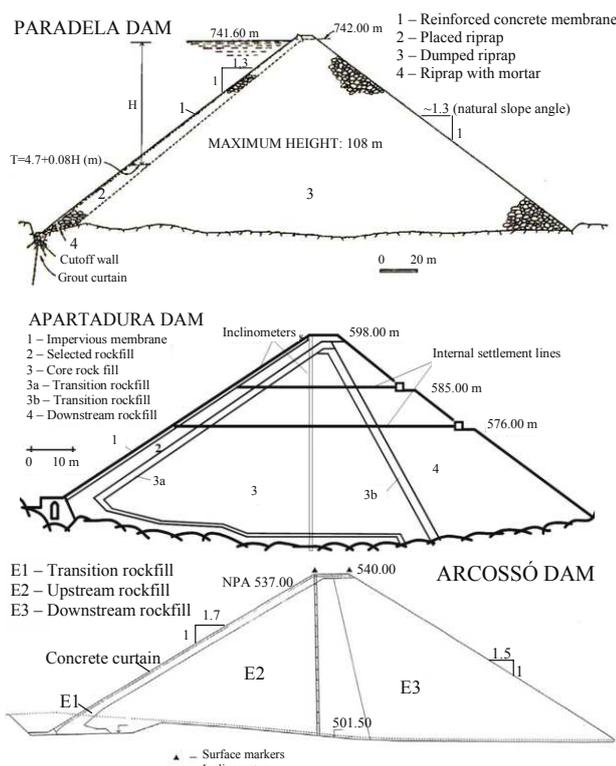
Figure 1. Cross-sections of some of the dams
