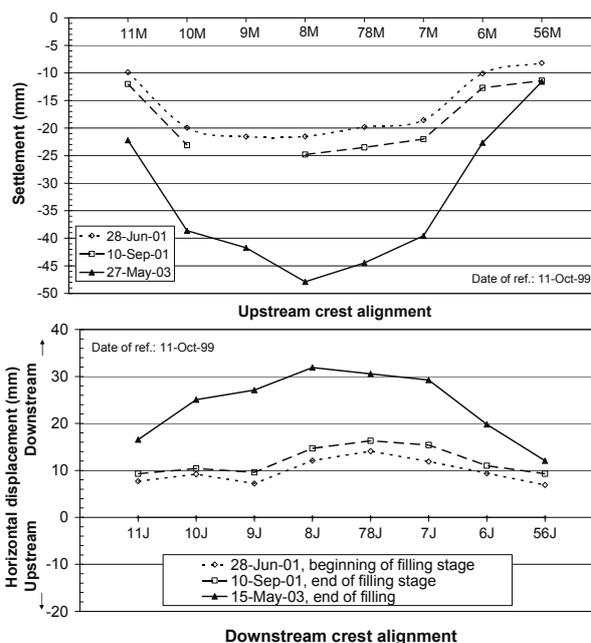
Figure 3. Arcossó Dam. Crest settlement and crest upstream-downstream horizontal displacement during first filling of the reservoir
