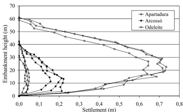
Figure 2. Internal settlements measured in vertical inclinometer tubes during embankment construction
