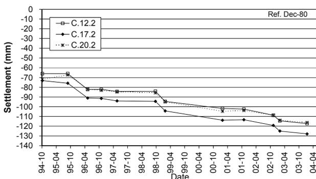
Figure 5. Paradela dam. Crest settlements versus time, at central marks
