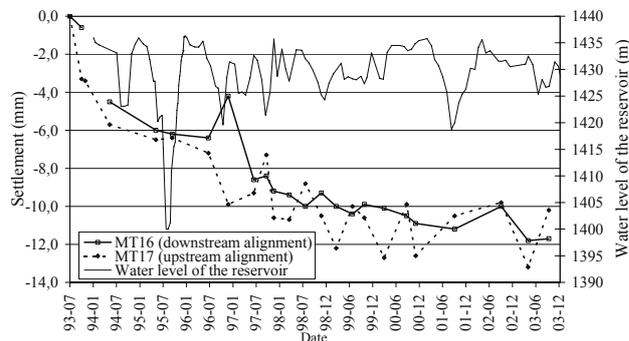
Figure 6. Lagoacho Dam. Crest settlements measured at the upstream and the downstream alignments since the end of the first filling
