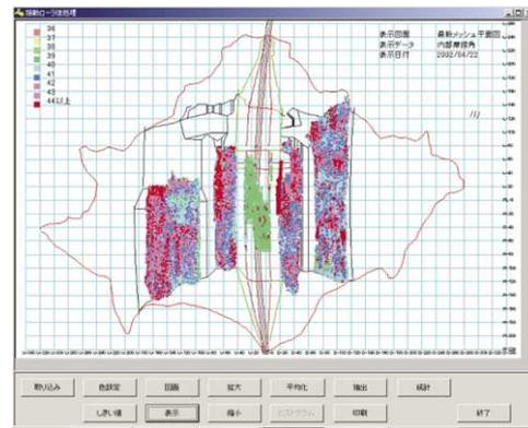
Figure 7. A two-dimensional distribution of internal friction angles at a certain elevation
