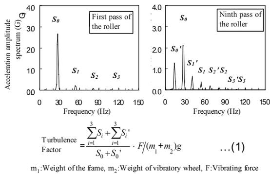
Figure 3. Fourier transform analysis of acceleration and definition of turbulence factor
