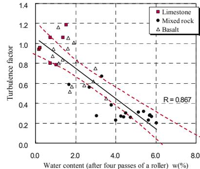
Figure 5. Water content and turbulence factor on roller compacted surface
