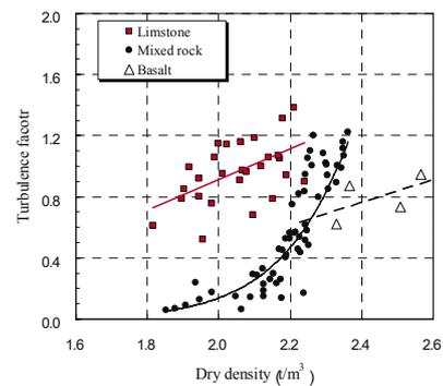
Figure 4. Dry density and turbulence factor of each material
