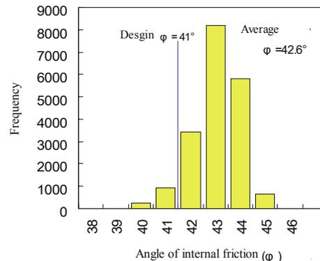
Figure 8. Histogram of the angle of internal friction
