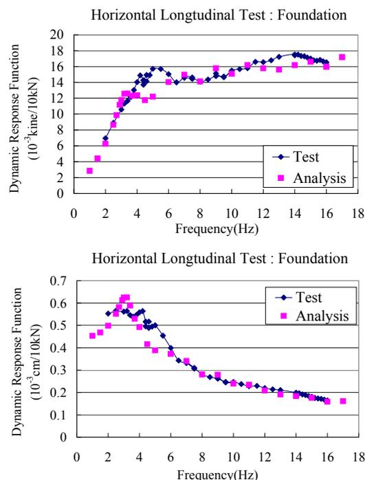
Figure 7. Dynamic response function in x-direction in horizontal longitudinal test (top: velocity; bottom: displacement).
