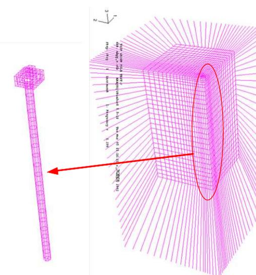
Figure 6. The FEM mesh used in numerical analysis.
