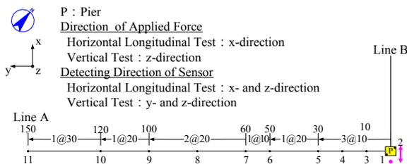
Figure 2. Layout of measuring points during the test.
