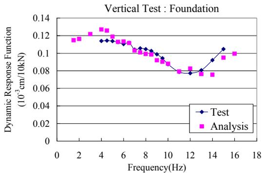
Figure 8. Dynamic response function in z-direction in vertical test (top: velocity; bottom: displacement).
