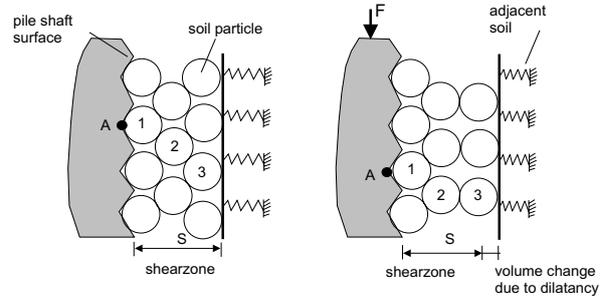
Figure 5. Pile-soil interaction, shearzone detail
