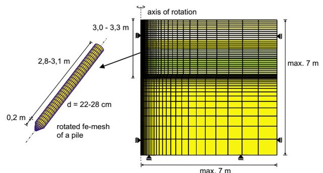
Figure 3. Axisymmetric FE-model
