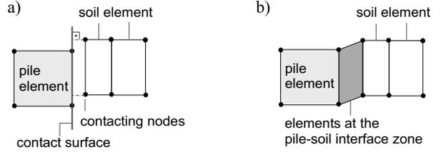
Figure 6. FE-modelling of pile-soil interaction zone (shearzone)
