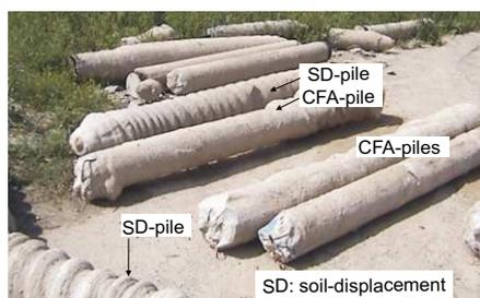
Figure 2. Excavated test piles after loading tests
