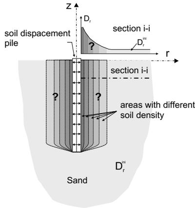
Figure 8. Assumed distribution of relative densities around a soil displacement pile
