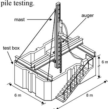
Figure 1. Setup for small scale testing of CFA-piles and soil-displacement piles (screwed piles)
