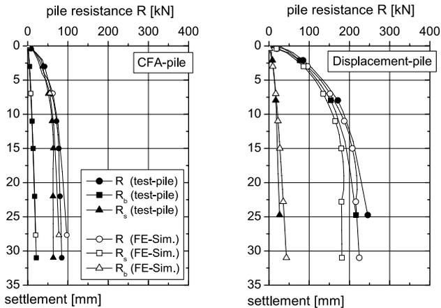
Figure 10. Comparison FE-Simulation and test pile behaviour (R: pile resistance,  $R_b$ : base resistance,  $R_s$ : shaft resistance)
