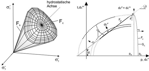
Figure 4. Drucker-Prager/Cap yield surfaces in the principal stress state and in the deviatoric stress plane
