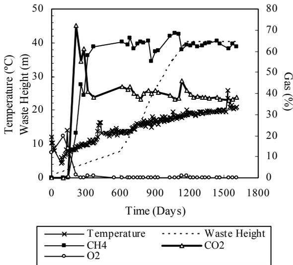
Figure 5. Gas composition and temperature for liner.
