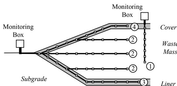
Figure 1. Schematic of temperature and gas monitoring points.
