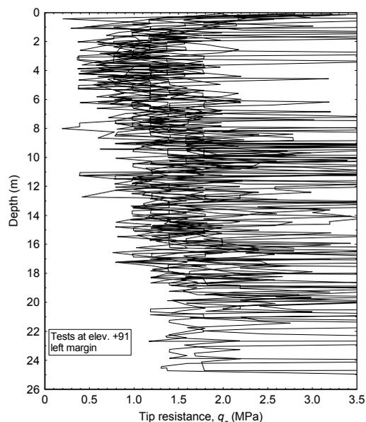
Figure 5. CPT tests on old mine fill before construction of the dam
