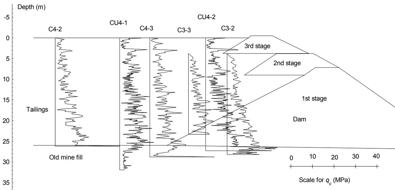
Figure 6. Tip resistance in CPT in tailings. Section 2-2.
