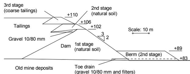
Figure 2. Dam cross-section at profile S-2
