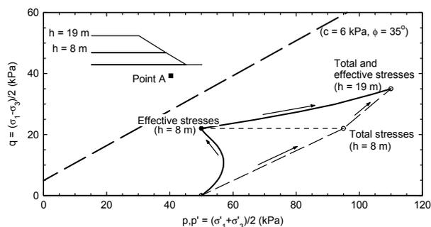
Figure 7. Typical stress paths below the toe of the dam
