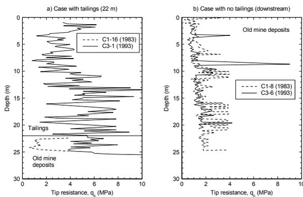
Figure 8. Example of cases with and without tailings surcharge
