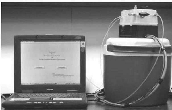
Figure 2. The portable electronic nose system
