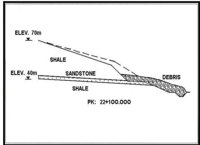
Figure 3 Channel Chongón – Playas, 22 Km., Ecuador. Slope failure adjacent to the channel, during El Niño 1997 – 1998.
