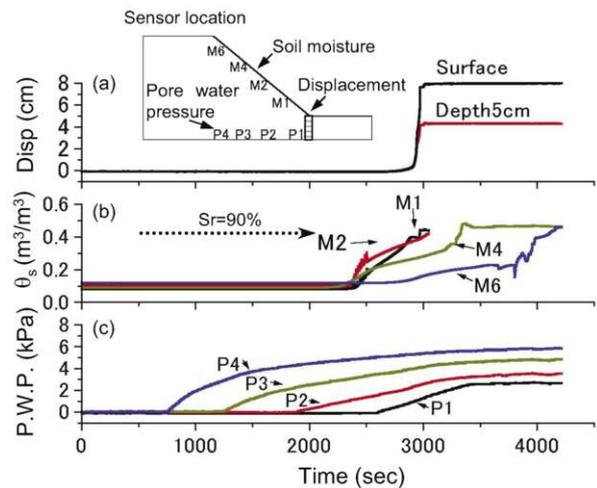
Figure 5. Time histories of: (a) toe displacement; (b) volumetric water content; (c) pore-water pressure at sensor locations (Case 1: seepage test)
