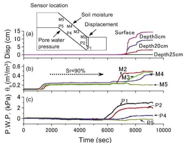
Figure 6. Time histories of: (a) toe displacement; (b) volumetric water content; (c) pore-water pressure at sensor locations (Case 2: rainfall test)
