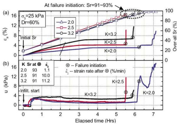
Figure 4. Time histories of: (a) axial strain,  $\epsilon_s$ , and over-all degree of saturation,  $S_r$ ; (b) pore water pressure,  $u$ , showing the effect of principal stress ratio,  $K$
