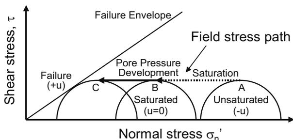
Figure 1. Field stress path in a slope subjected to rainwater infiltration
