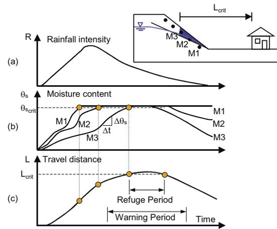
Figure 8. Schematic diagram showing the time histories of: (a) rainfall,  $R$ ; (b) moisture content,  $\theta_s$ ; (c) travel distance,  $L$
