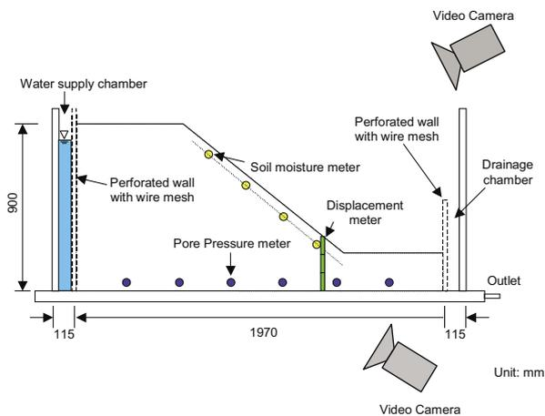
Figure 2. Schematic diagram of the soil box and the sensor locations
