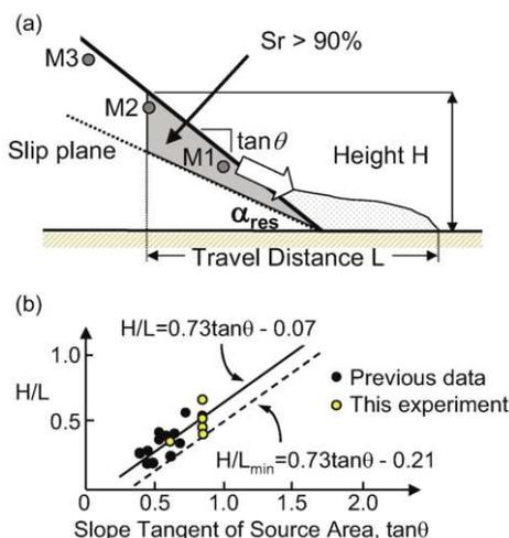
Figure 7. Basis of monitoring scheme: (a) zone with high potential for sliding; (b) relation between  $H/L$  and slope tangent of slide source area
