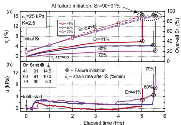
Figure 3. Time histories of: (a) axial strain,  $\epsilon_a$ , and over-all degree of saturation,  $S_r$ ; (b) pore water pressure,  $u$ , showing the effect of varying relative density,  $Dr$
