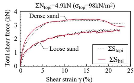
Figure 4. Total shear forces on the top and bottom planes of a specimen
