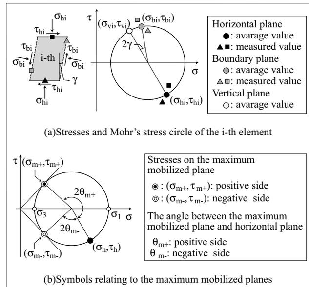
Figure 3. Determination of Mohr's stress circle and symbols relating to the maximum mobilized planes
