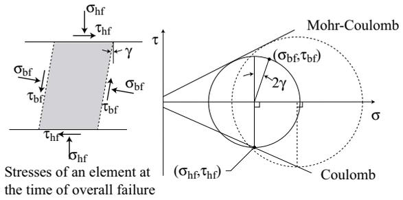
Figure 12. The relation between Coulomb's and Mohr-Coulomb's failure criteria
