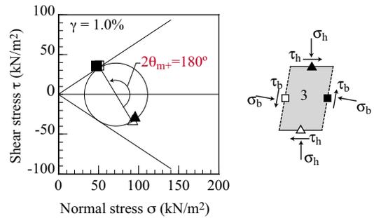
Figure 8. Mohr's stress circle at  $\gamma = 1\%$  (the central element 3)
