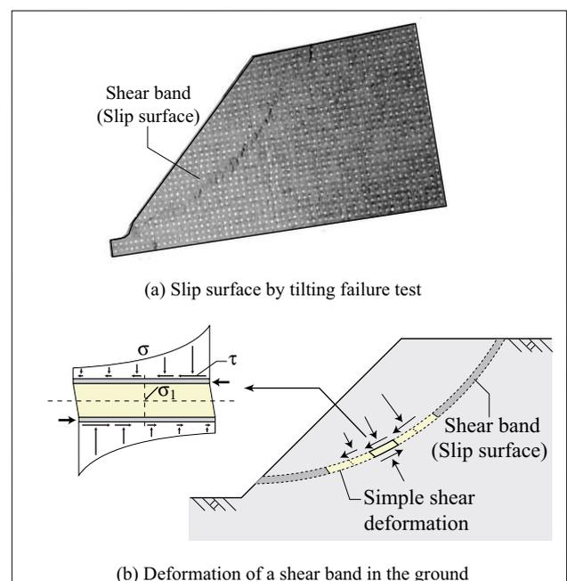
Figure 1. Slip surface and shear band
