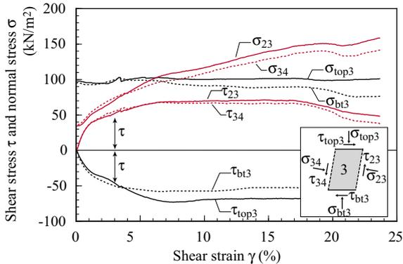
Figure 6. Changes of the stresses acting on the central element
