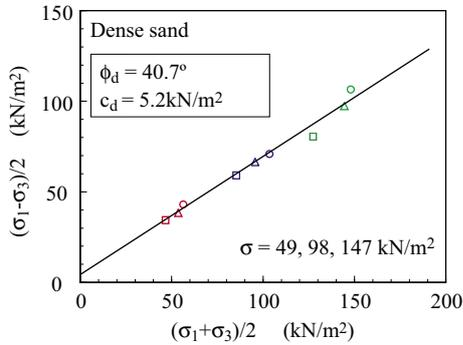
Figure 10. Mohr-Coulomb's failure criterion (dense sand)
