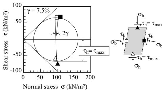
Figure 11. Mohr's stress circle at the time of overall failure of  $\gamma=7.5\%$  (the central element)
