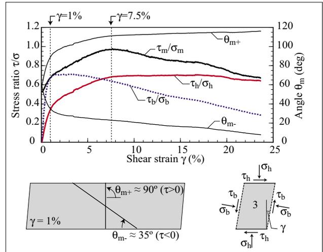
Figure 7. Changes of stress ratios and the angles between the maximum mobilized planes and horizontal plane of the central element
