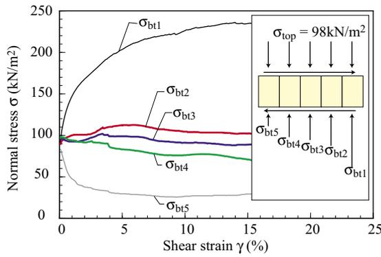
Figure 5. Normal stresses acting on the bottom planes of soil elements
