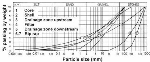
Figure 2. Average grain size distribution curves of dam materials
