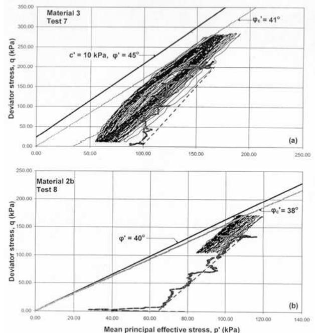
Figure 5. Anisotropic consolidation followed by cyclic loading at 0.1 Hz: (a) Material 3, Test 7; (b) Material 2b, Test 8
