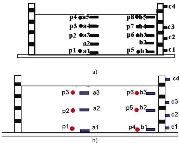
Figure 1. Instrumentation layout for a) BT-4 and b) BT-10.
