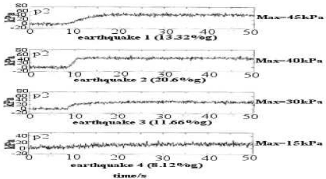
Figure 5. Excess pore pressure results for test BT-4 (after Teymur and Madabhushi, 2003).
