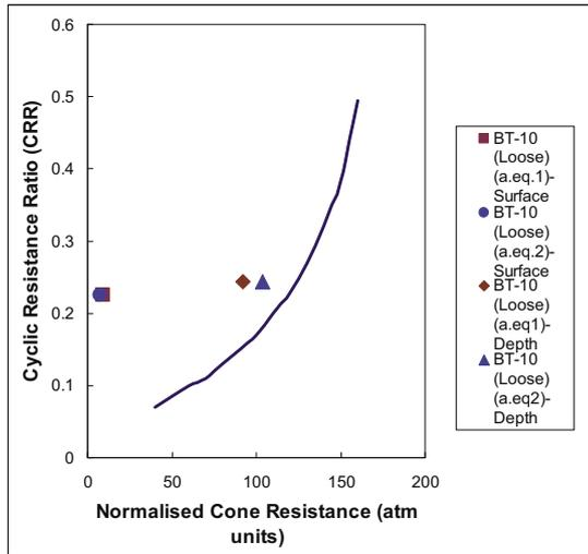
Figure 2. Liquefaction assessment of centrifuge data at the centre of the soil model after the earthquake. (Teymur, 2002)
