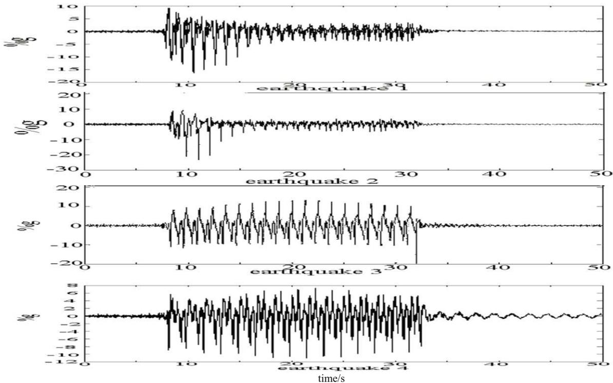
Figure 6. Acceleration histories for test BT-4
