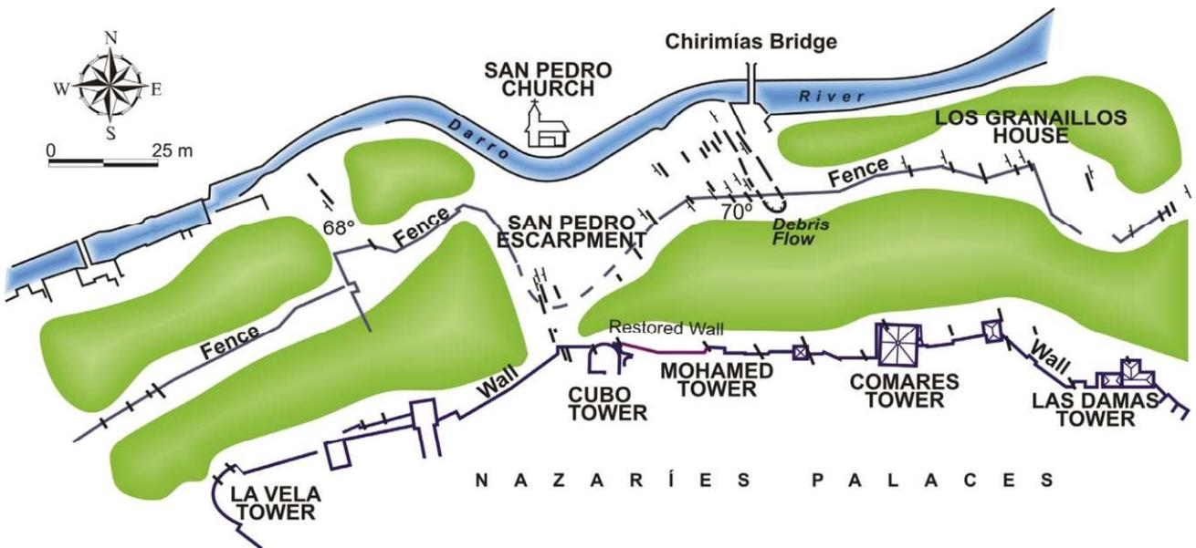
Figure 2. Outline of the site showing the main cracks at *La Alhambra* fence and wall and faults at the hill slope.
