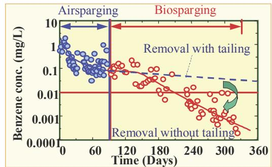
Figure 5. Effect of Air/Bio sparging at this site
