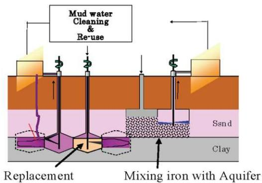
Figure 3. Application of Jetting Method for in-situ remediation
