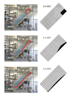
Figure 4. Experiment and simulation for granular flow
