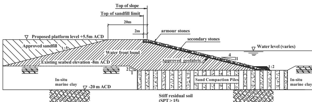
Figure 1 Typical water front bund design scheme
