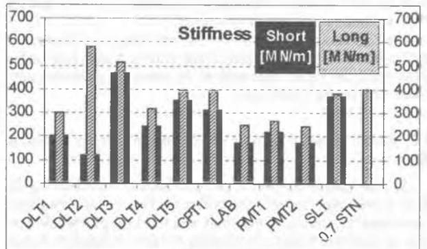
Figure 7 : Stiffness distribution for long and short piles.
