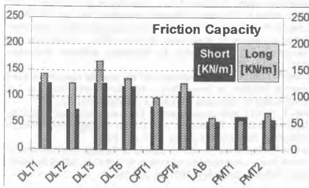
Figure 5 : Friction Capacity distribution for long and short Precast piles.
