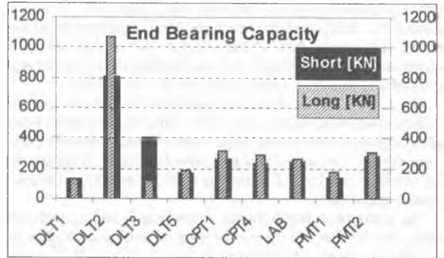
Figure 6 : End Bearing Capacity distribution for long and short Precast
