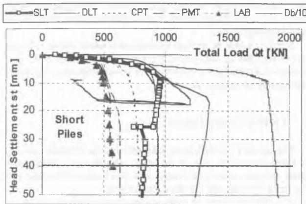
Figure 3 : Predictive Qt comparison of short piles
