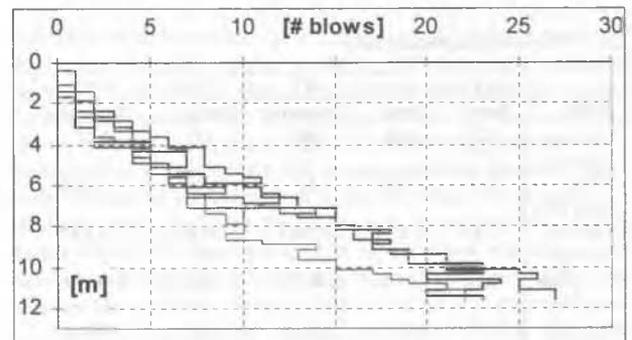
Figure 1 : Blow count diagram of Precast Pile per 25 cm penetration.
