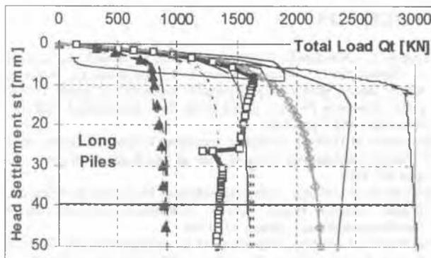
Figure 4 : Predictive Qt comparison of long piles.
