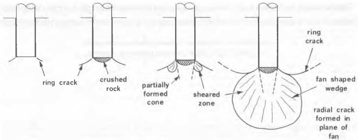
Figure 1 Failure processes around pile tip
