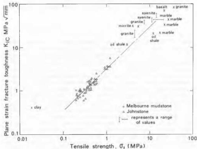
Figure 6 Relationship between plane strain fracture toughness and tensile strength for some rocks and soils
