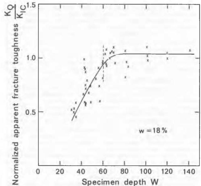
Figure 4 Influence of beam depth on fracture toughness
