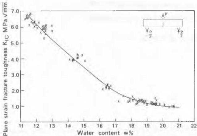
Figure 5 Variation of plane strain fracture toughness of Johnstone with saturated water content
