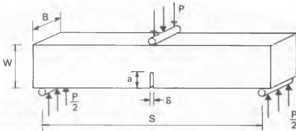
Figure 3 Test arrangement of three point loading of single edge cracked beams
