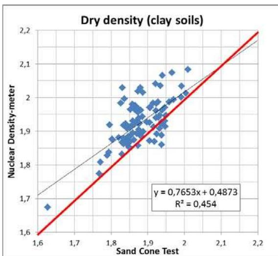
Fig. 3 Nuclear density-meter vs sand cone tests results for the dry density in clay soils with corrections.
