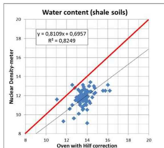
Fig. 5 Nuclear density-meter vs sand cone tests results for the water content in shale soils.
