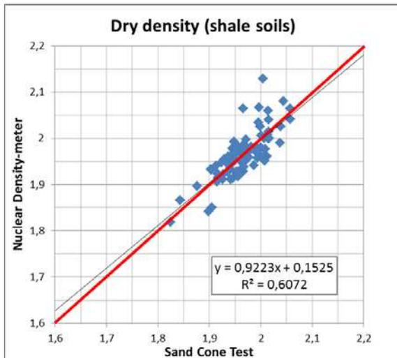
Fig. 6 Nuclear density-meter vs sand cone tests results for the dry density in shale soils.
