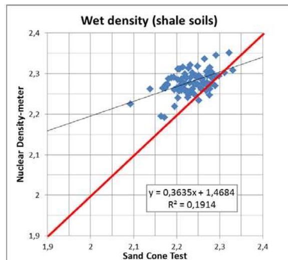
Fig. 4 Nuclear density-meter vs sand cone tests results for the wet density in shale soils.
