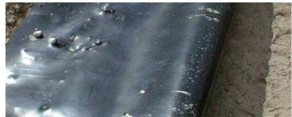
Fig. 4 Geomembrane damaged by stones in an unsuitable foundation (Photo: courtesy of R. Thiel)
