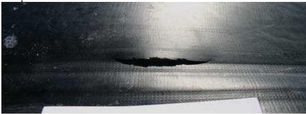
Fig. 9 Defect on underside of a geomembrane weld that would not be detected by an air channel test or casual visual inspection from the top of the geomembrane
