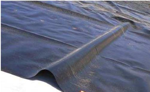
Fig. 1 HDPE geomembrane with a wrinkle
