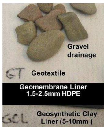
Fig. 3 Typical barrier with gravel drainage layer, geotextile protection layer, HDPE geomembrane, and GCL
