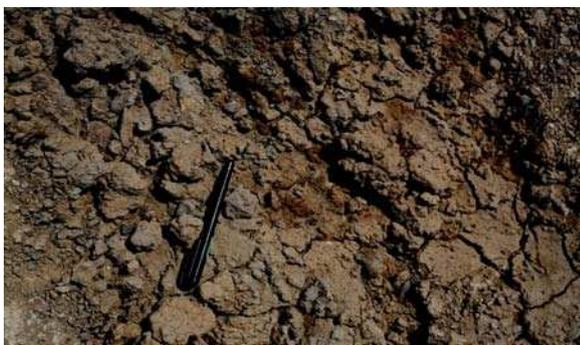
Fig. 6 Eroded foundation layer due to heavy rainfall
