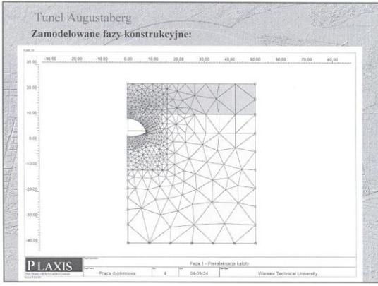
Figure 5. Finite element mesh – PLAXIS.
