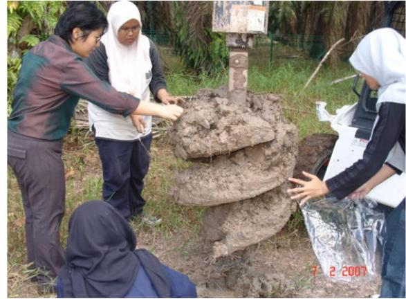
Figure 1. Retrieval of clay sample.
