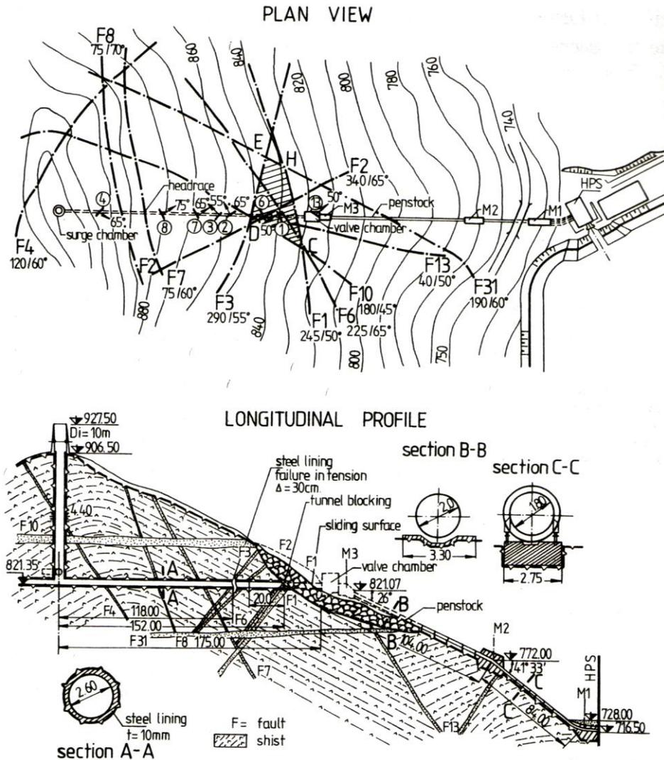
Figure 6. Hydraulic circuit of Leresti powerplant: site geology and affected works
