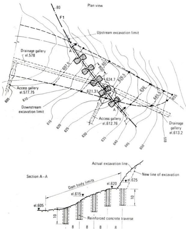
Figure 5. Fault consolidation by concrete traverses.
