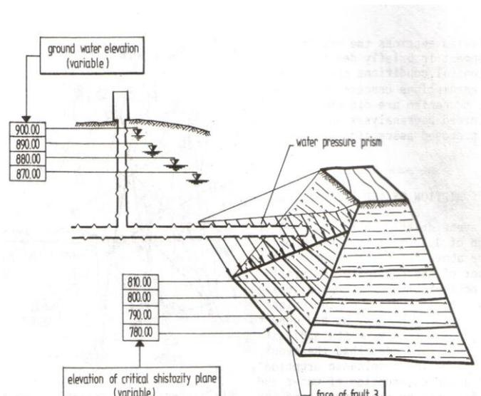
Figure 8. The computational model of the pressure forces
