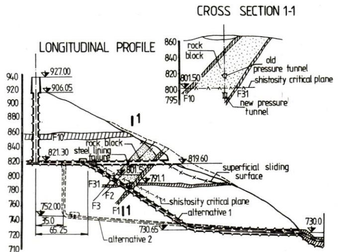
Figure 9. Alternatives for reconstruction of a new water circuit downstream of surge tank.
