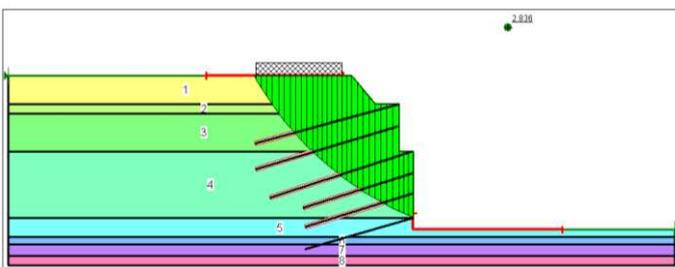
Figure 1. Engineering Geological Applications in Building Construction course, Laboratory based practical sessions. An example of slope stability analysis and the proposed solution with the calculated factor of safety (2.8).
