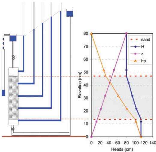
Figure 6. Diagram of permeameter showing the variation of total, pressure and elevation heads for one flow rate.
