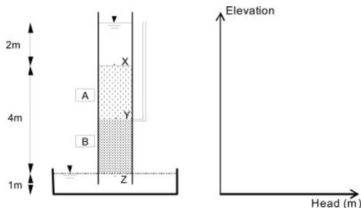
Figure 3. Problem to calculate and draw the variation of total head, pressure head and elevation head down the centre-line of a large tube containing two layers of sand A and B when i)  $k_A = k_B$  and ii)  $k_A = 2 * k_B$ .
