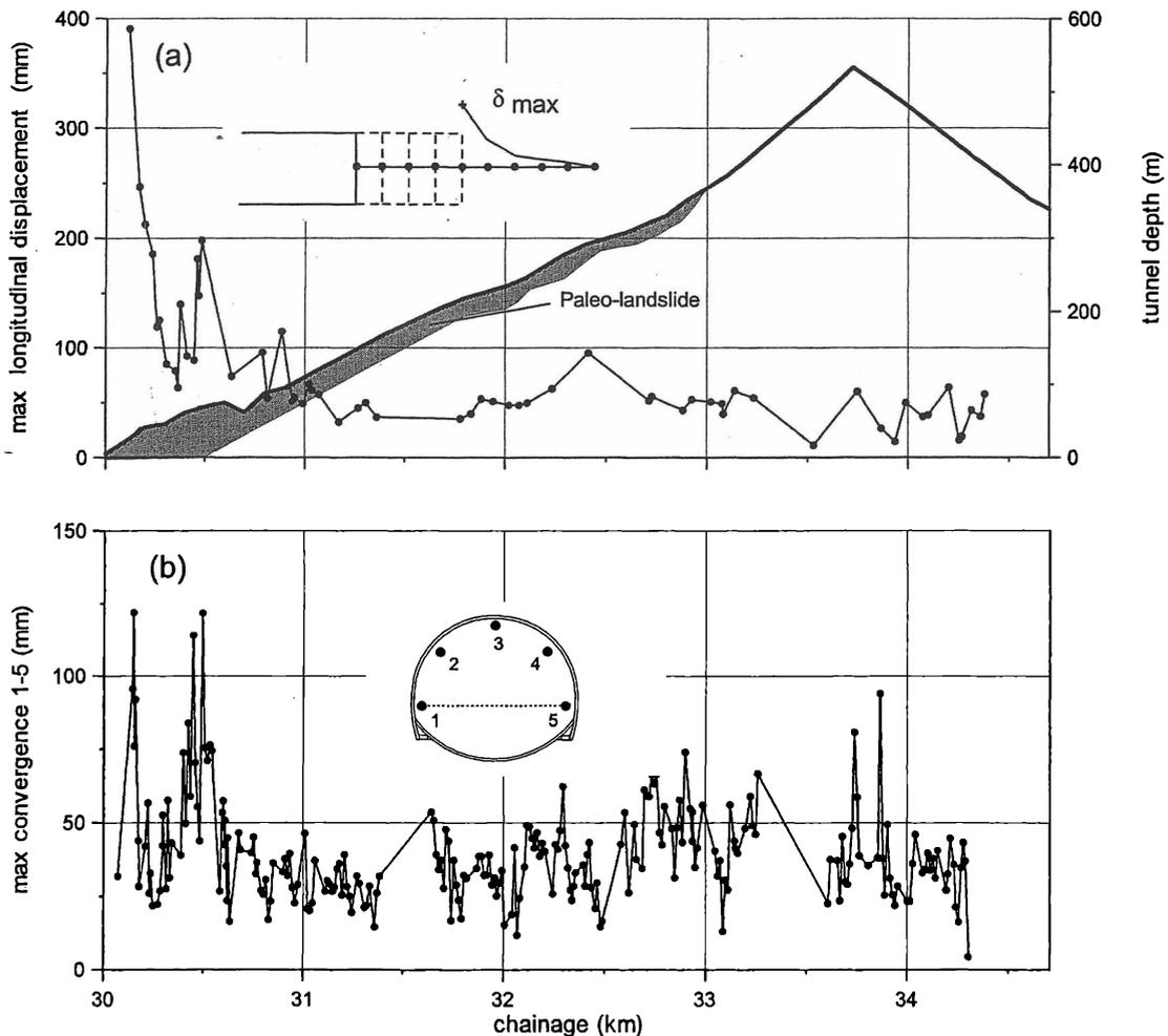
Figure 5. Profile of maximum values of convergence and extrusion measured along the tunnel route.
