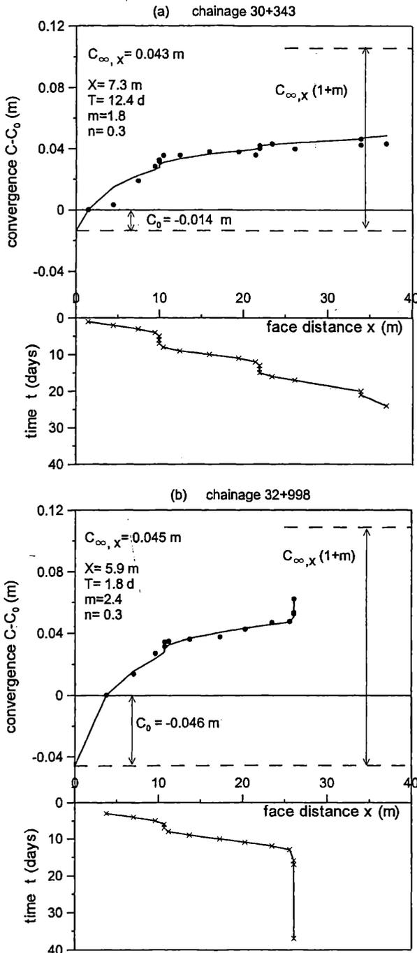
Figure 6. Curve fitting of convergence measurements at two monitoring sections.
