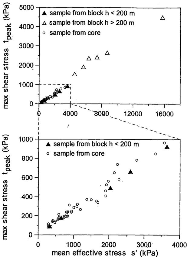
Figure 2. Synopsis of laboratory peak strength measurements of clay shale samples.
