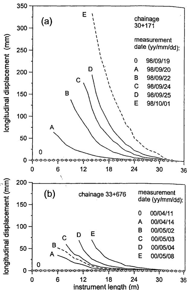
Figure 4. Longitudinal displacements ("extrusion") measured during face advance along a pipe installed at two different chainages.
