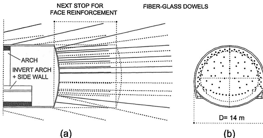
Figure 3. Cross-section of the tunnel and longitudinal profile.
