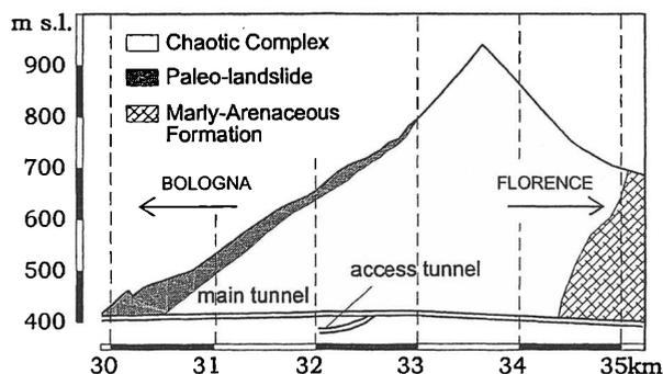
Figure 1. Geological profile along the tunnel route.
