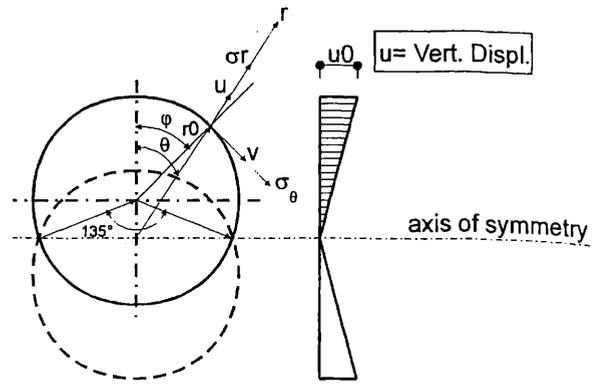
Figure 8: Embedment of  $135^\circ$ ; stresses on the lining and vertical ground displacements.
