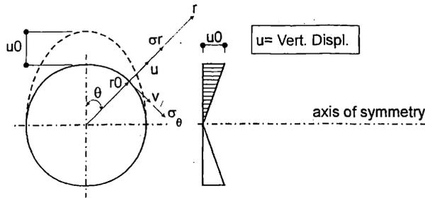
Fig 7: Embedment of  $180^\circ$ ; stresses on the lining and vertical ground displacements.
