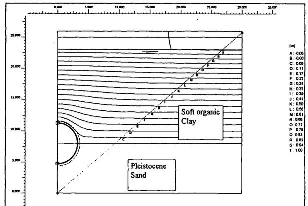
Figure 9: Contour lines vertical displacements around tunnel tube.
