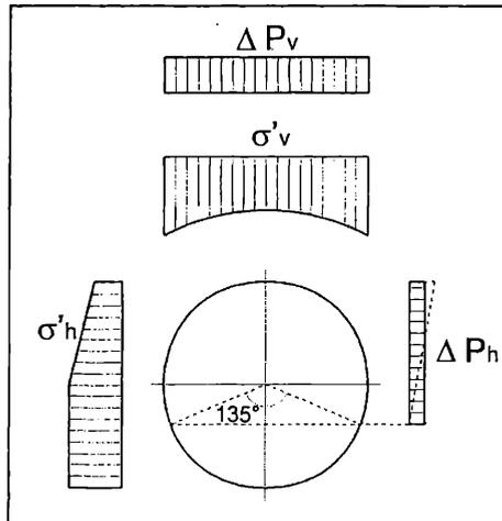
Figure 6: Loading scheme on the lining;  $\Delta p_v$  and  $\Delta p_h$  are the extra loading stresses due to long term settlements.
