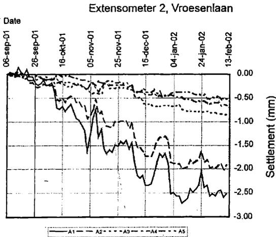
Figure 4: Extensometer measurements. Horizontal axis; time. Vertical axis; settlement in mm.
