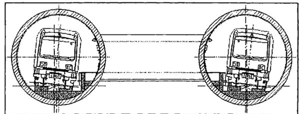
Figure 1: Two single-track tunnels of 6.5 m diameter.
