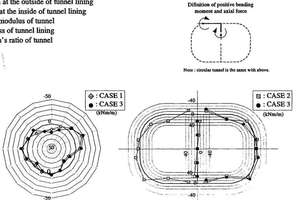
Figure 4. Bending moment at the centrifugal acceleration 50G (: initial).
