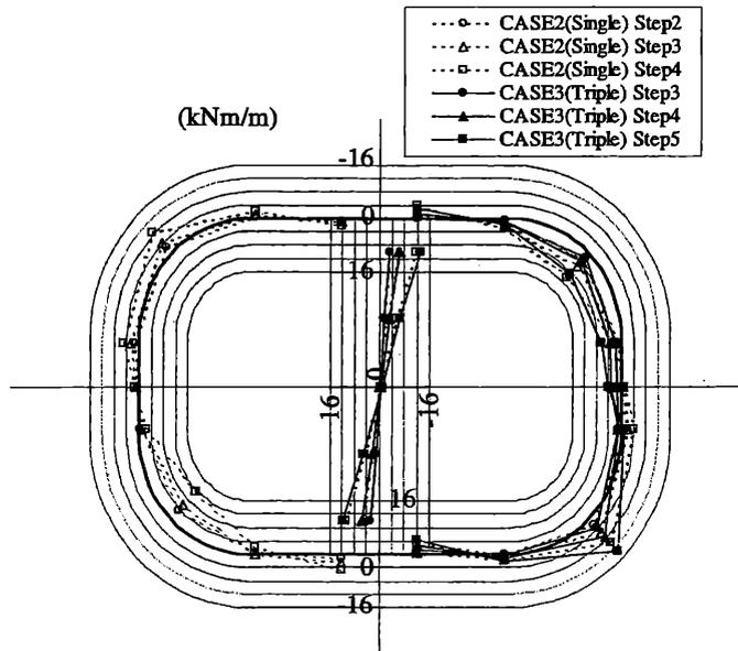
Figure 9. Comparison between single tunnel and triple-faced tunnel (bending moment) for approximately same displacement.
