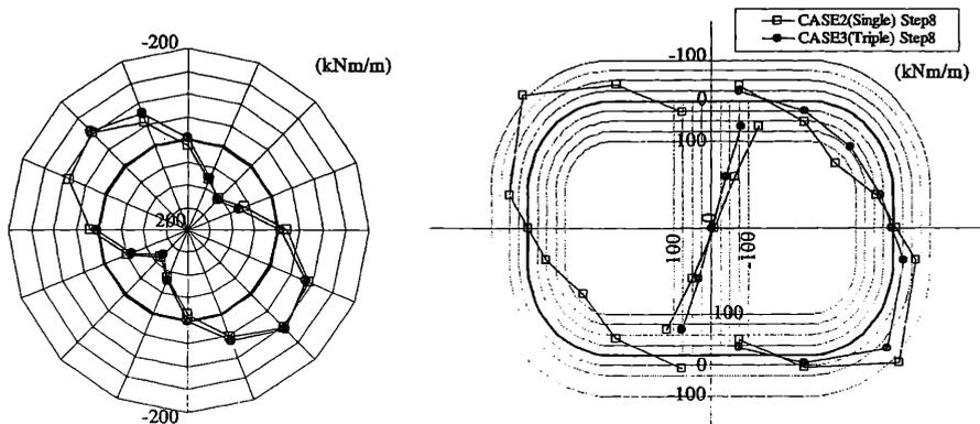
Figure 8. Comparison between single tunnel and triple-faced tunnel (bending moment).
