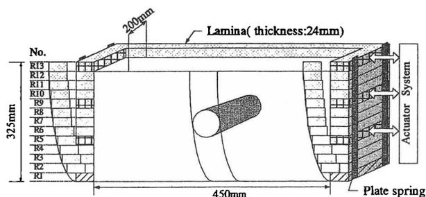
Figure 1. View of the shear box.
