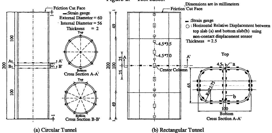
Figure 3. Outline of tunnel models and measurements.
