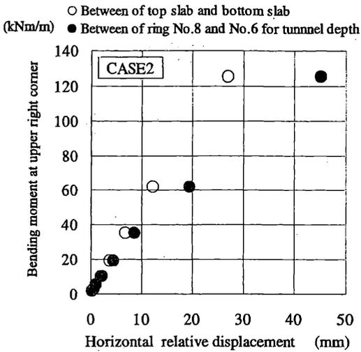
Figure 7. Relationship between bending moment and horizontal relative displacement
