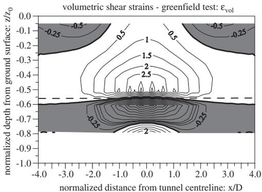
Figure 6. Greenfield test: contours of volumetric strain, compression is positive ( $V_L = 20.0\%$ ).
