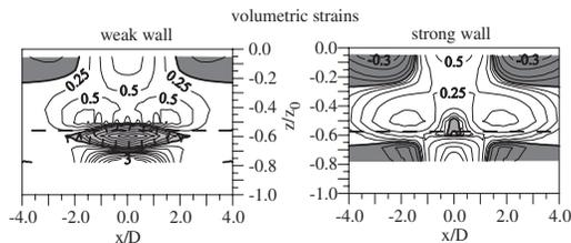
Figure 7. Wall-ground interaction tests: contours of volumetric strains ( $V_L = 20.0\%$ ).
