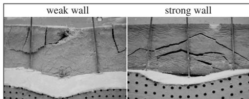
Figure 9. Failure mechanism of model-walls tested.
