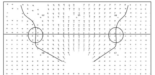
Figure 5. Ground displacement vectors around the tunnel.
