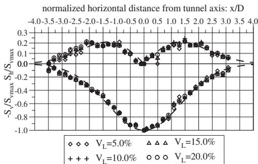
Figure 2. Typical experimental data from centrifuge testing and their interpolation by cross-hatched lines: normalized distance from tunnel axis ( $x/D$ ) against normalized horizontal displacement ( $S_h/S_{vmax}$ ) and vertical displacement ( $-S_v/S_{vmax}$ ).
