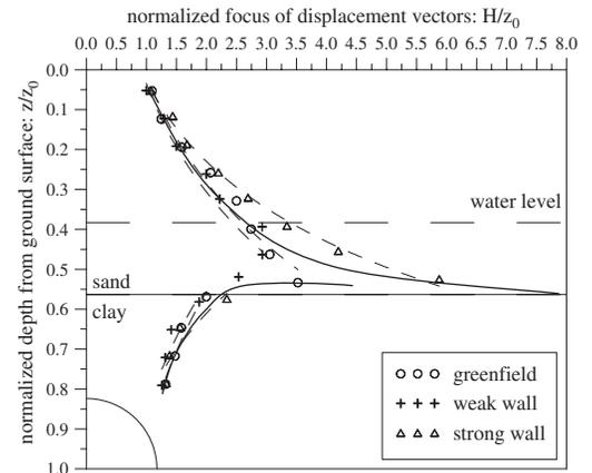
Figure 4. Normalized focus of displacement vectors ( $H/z_0$ ) against normalized depth from ground surface ( $z/z_0$ ).
