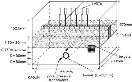
Figure 1. Schematic of centrifuge model.
