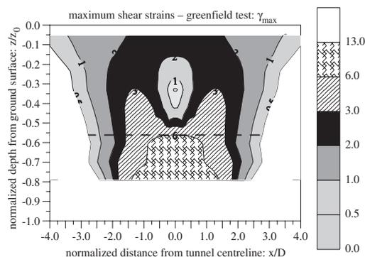
Figure 8. Greenfield test: contours of maximum shear strain ( $V_L = 20.0\%$ ).
