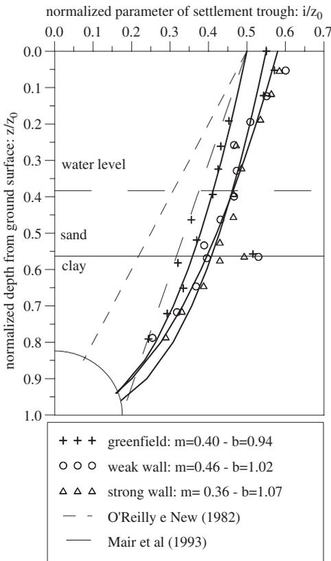
Figure 3. Normalized parameter of settlement trough ( $i/z_0$ ) against normalized depth from ground surface ( $z/z_0$ ).
