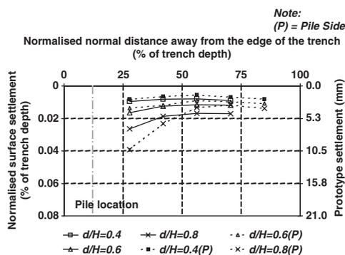
Figure 9. Normalised surface settlement ( $\Delta/H$ ) along the centre-line of the trench (40 mm) at different relative drop in slurry level ( $d/H$ ) for case with  $x/D = 3.5$ .
