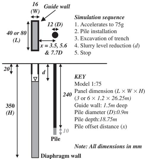
Figure 1. Geometry of test set-up and summary of the values changed in the centrifuge tests.
