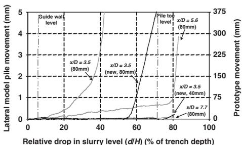
Figure 5. Variation of lateral movements at head of piles installed at different normalised distances from the edge of the trench ( $x/D$ ) with relative drop in slurry level ( $d/H$ ).
