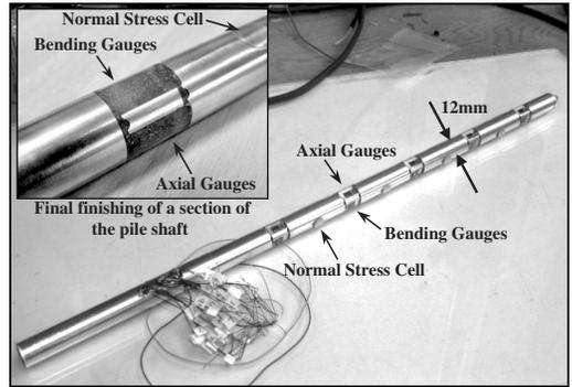
Figure 2. Measuring units of the new version instrumented model pile.
