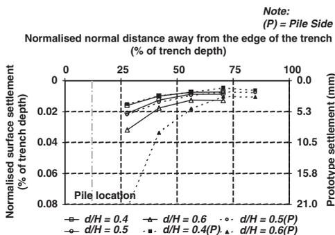
Figure 8. Normalised surface settlement ( $\Delta/H$ ) along the centre-line of the trench (80 mm) at different relative drop in slurry level ( $d/H$ ) for case with  $x/D = 3.5$ .
