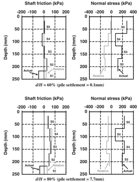
Figure 7. Shaft friction and normal stress distributions of a pile installed at  $x/D = 3.5$  with different drops in slurry level ( $d/H$ ) (40 mm trench).
