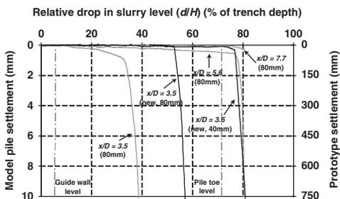
Figure 4. Variation of settlements at head of piles installed at different normalised distances from the edge of the trench ( $x/D$ ) with relative drop in slurry level ( $d/H$ ).
