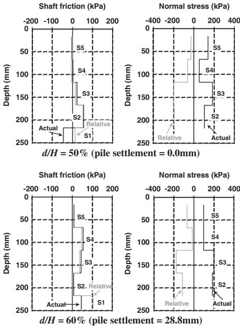
Figure 6. Shaft friction and normal stress distributions of a pile installed at  $x/D = 3.5$  with different drops in slurry level ( $d/H$ ) (80 mm trench).
