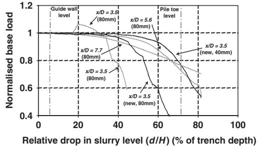
Figure 3. Variation in normalised base load ( $Q_{bn}$ ) on piles installed at different normalised distances from the edge of the trench ( $x/D$ ) with relative drop in slurry level ( $d/H$ ).
