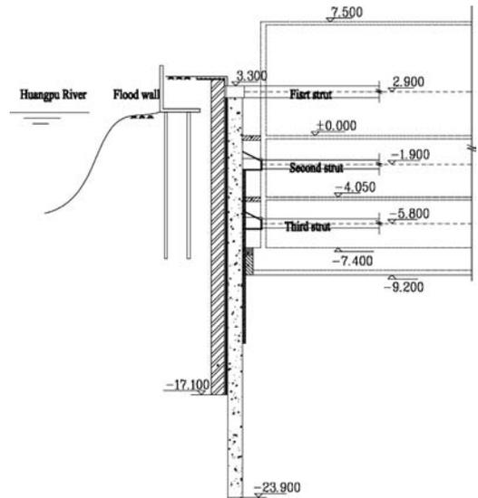
Figure 3b. B-B cross section of deep excavation.
