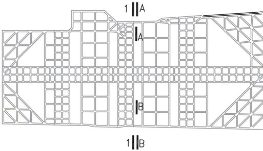
Figure 2. The plane view of strut arrangement.
