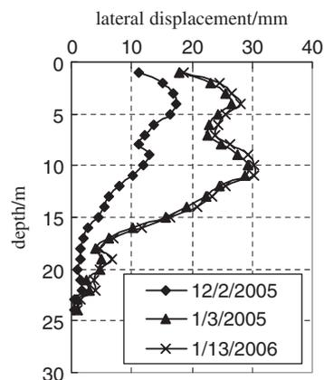
Figure 6. Lateral displacement at inclinometer CX12.
