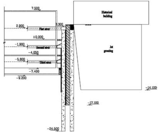
Figure 3a. A-A cross section of deep excavation.
