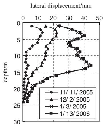
Figure 5. Lateral displacement at inclinometer CX1.
