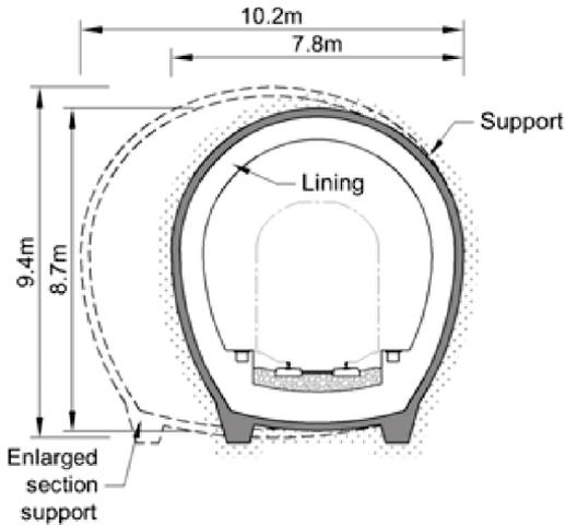
Figure 1. Type profiles (basic and enlarged cross-sections).
