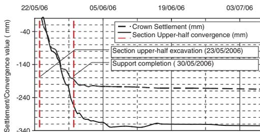
Figure 6. Greatest tunnel deformations, measured at PK 26+978.
