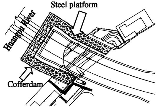
Figure 10. The cofferdam and steel platform in the Huangpu River.
