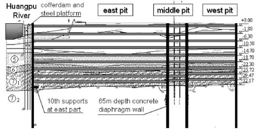
Figure 4. Ground profile at the restoration project site.
