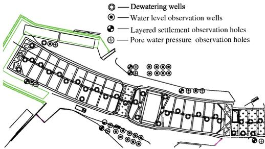
Figure 12. Dewatering monitoring points of the eastern pit.
