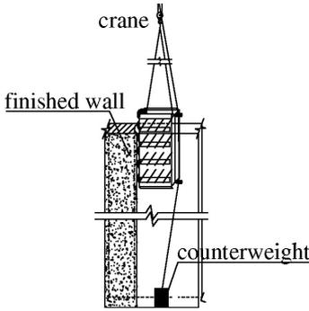
Figure 9. Brushing work for the diaphragm wall.
