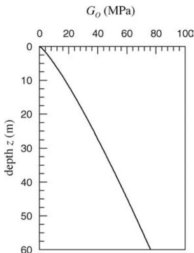
Figure 3. Profile of the small-strain shear stiffness  $G_0$ .
