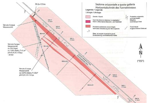
Figure 8. Plan of investigated fault zone and water ingress at TM 6000 to 6150.
