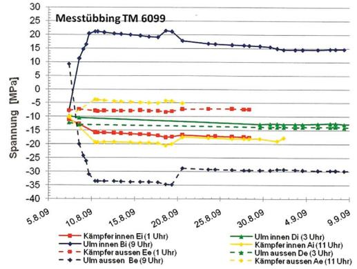
Figure 6. Data from the measurement segment at TM 6099.
