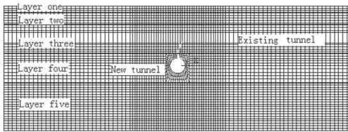
Figure 5. Finite element mesh for five layered soils.
