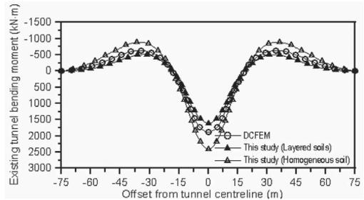
Figure 8. Comparisons of existing tunnel bending moment.
