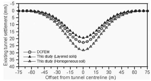
Figure 7. Comparisons of existing tunnel settlement.
