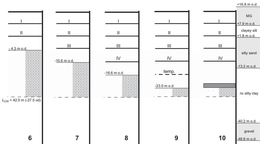
Figure 2. Excavation stages; cross-wall length  $L_{\text{cw}} = 42.5$  m.
