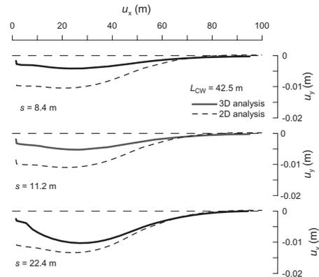
Figure 10. Surface settlement profiles computed by 3D and 2D analyses:  $L_{cw} = 42.5 \text{ m}$ ,  $s = 11.2 \text{ m}$ .
