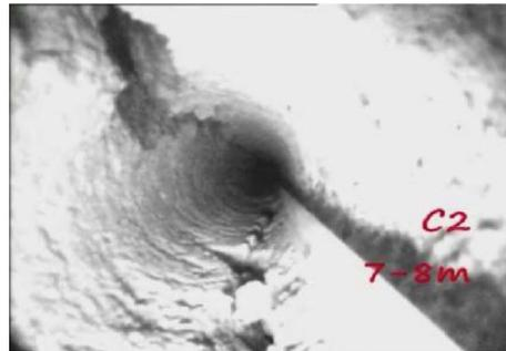
Figure 6. Borehole camera in corings, with evident fractures.
