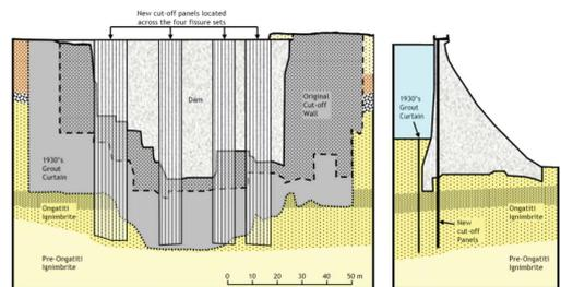
Figure 3. Arapuni cut-off wall (view and cross section).
