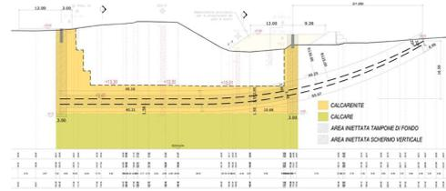
Figure 8. Bottom slab created by directional drilling.
