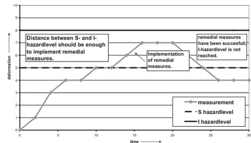
Figure 5. Principle of determining S- and I-hazard level.
