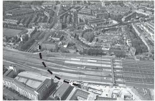
Figure 3. Location of bored tunnel under 13 railway tracks of Rotterdam Central Station.
