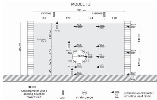
Figure 9. Layout of the model T3.
