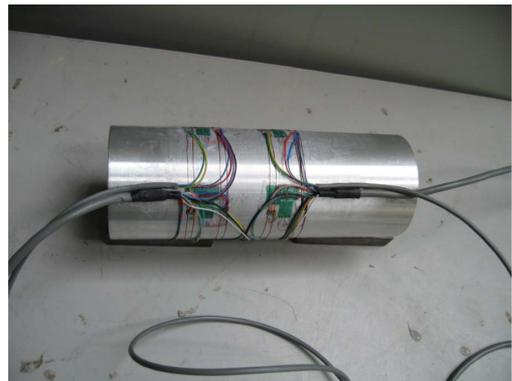
Figure 5. Instrumented tube.
