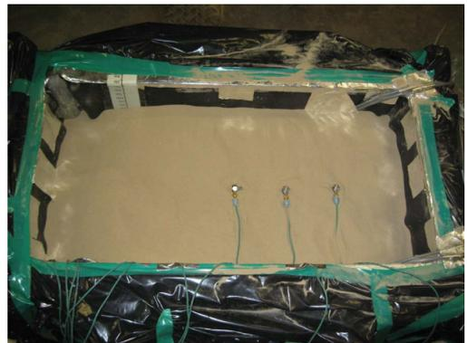
Figure 6. Accelerometers positioning.
